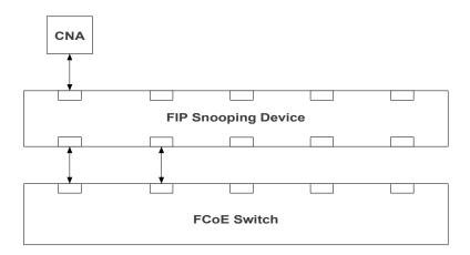
**Test Setup 2:** The Initiators are connected to the FIP Snooping Device. The The FIP Snooping Device is then connected to the FCoE Switch.
