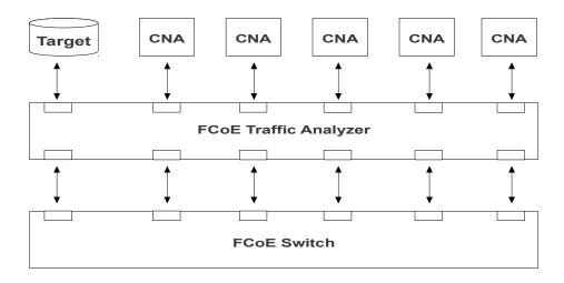
**Test Setup 3:** The Targets and the Initiator are connected to the analyzer. The Targets are then connected in a fabric with the Initiator through the Switch.
