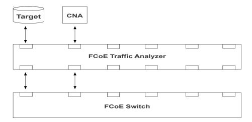
**Test Setup 2:** The Target and the Initiators are connected to the analyzer. The Target is then connected to the Initiators through the Switch.
