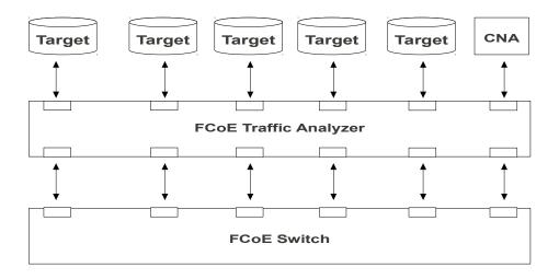
Test Setup 4: Multiple Targets and multiple Initiators are connected to the fabric through the Switch.
