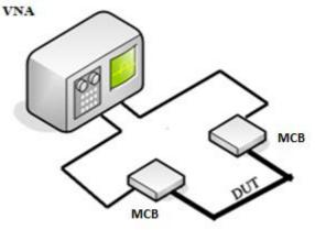
The VNA is setup so that differential port 1 is connected to the TX side of one card while differential port 2 is attached to the RX side on the other card.
