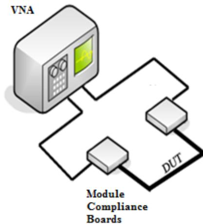
The DUT is connected between two module compliance boards. The VNA is connected to the victim transmit pair on one MCB and the victim receive pair on the other. The VNA shall be properly calibrated before use.
