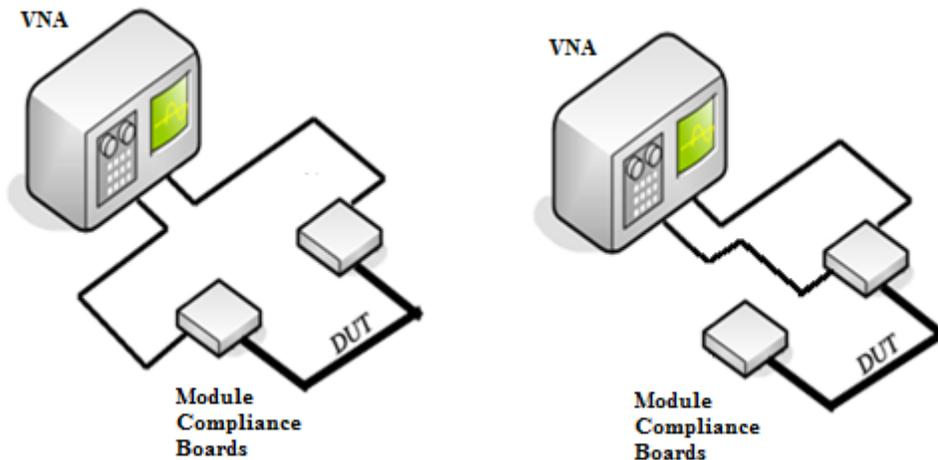
The DUT is connected between two module compliance boards. In order to test near-end crosstalk the VNA is connected to the victim receive pair on one MCB and to all transmit pairs on the same MCB. In order to test far-end crosstalk the VNA is connected to the victim receive pair of one MCB and to each non-victim transmit pair on the other MCB. The VAN shall be properly calibrated before use.
