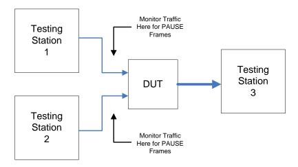
For an end station, the DUT may require a long period of time to reply to frames. Valid frames transmitted at minimum interPacketGap could fill the buffers of the DUT, forcing it to transmit PAUSE frames. Another option for filling the DUT's buffers is to send frames separated by less than minimum IPG or to send frames with less than seven bytes of preamble. These options are not, however, supported by all testing stations.
