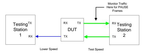
If the device has more than two ports, connect three of the ports to testing Stations. Have Testing Station 1 and Testing Station 2 transmit frames at line rate to Testing Station 3. The DUT will not be able to forward all the frames to Testing Station 3, so it may attempt to pause the transmission of Testing Station 1 and Testing Station 2.
