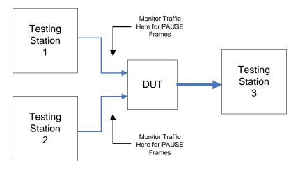
For an end station, the DUT may require a long period of time to reply to frames. Valid frames transmitted at minimum interframe gap could fill the buffers of the DUT, forcing it to transmit PAUSE frames. Another option for filling the DUT's buffers is to send frames separated by less than minimum IFG or to send frames with less than seven bytes of preamble. These options are not, however, supported by all testing stations.
