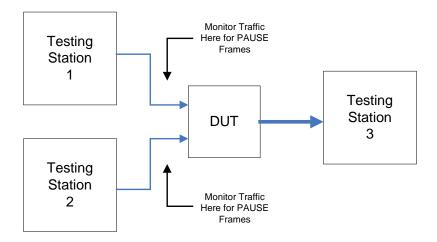
For an end station, the DUT may require a long period of time to reply to frames. Valid frames transmitted at minimum interframe gap could fill the buffers of the DUT, forcing it to transmit PAUSE frames. Another option for filling the DUT's buffers is to send frames separated by less than minimum IFG or to send frames with less than seven bytes of preamble. These options are not, however, supported by all testing stations.
