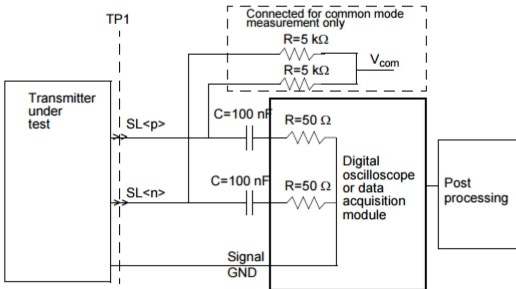
**128.A-1: example test setup for tests 128.1.1 through 128.1.7**
