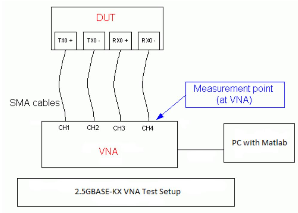
**128.A-2: example test setup for tests 128.2.1 through 128.2.3**
