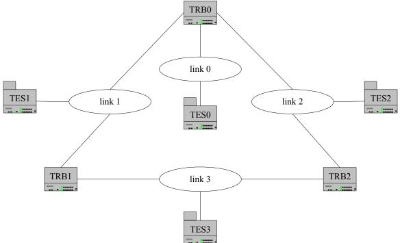
For ease of transition between test setups TRB1 and TRB2 should also be physically wired to link 0. TRB1's and TRB2's ports to link 0 should be disabled. All transmissions of multicast ethernet data in this test suite refers to non-IPv4 and non-IPv6 multicast ethernet data unless otherwise specified.
