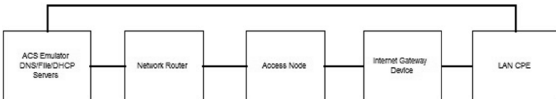
Figure 4: End Device Test Setup via Ethernet through an RG that is connected via DSL/PON/Cable
