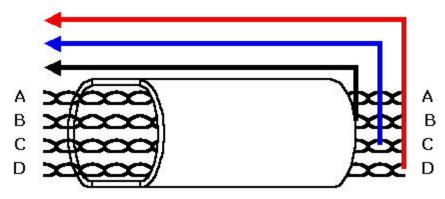
Crosstalk coupling between a local receiver and remote transmitters.
