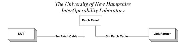
Use the DSP-4000 Fluke to make sure the connection is good (no crossover or broken link) and that the NEXT and NEXT-at-REMOTE (cross-talk) values pass. If the cross-talk values do not pass, make sure that the wires connecting from the top row to the bottom row are straight and don't touch other pairs or cross over with them. If they still fail, fiddle with the wire arrangement or start all over (this occurrence is rare, cross-talk usually passes over low attenuation).
