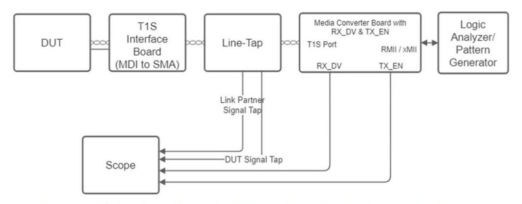
Some test cases could be performed simply from MII level observations of link partner signaling (including some simple PCS tests, MAC, Flow Control, etc) (Note, a "Link Status" from the "Media Converter / MII" board might be needed for some tests)
