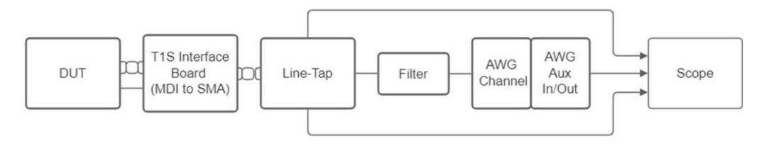
Most test cases can be performed with UNH-IOL developed MATLAB code to generate the required test signaling is provided to a suitable AWG with Filter as needed for PSD mask standards compliance.
