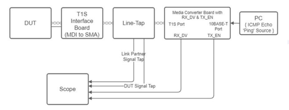
Some higher-level test cases can benefit from simpler setups with Media Converters and monitoring when needed – this can also include stressed receiver environment tests where packet error rate to estimate bit error rate is useful
